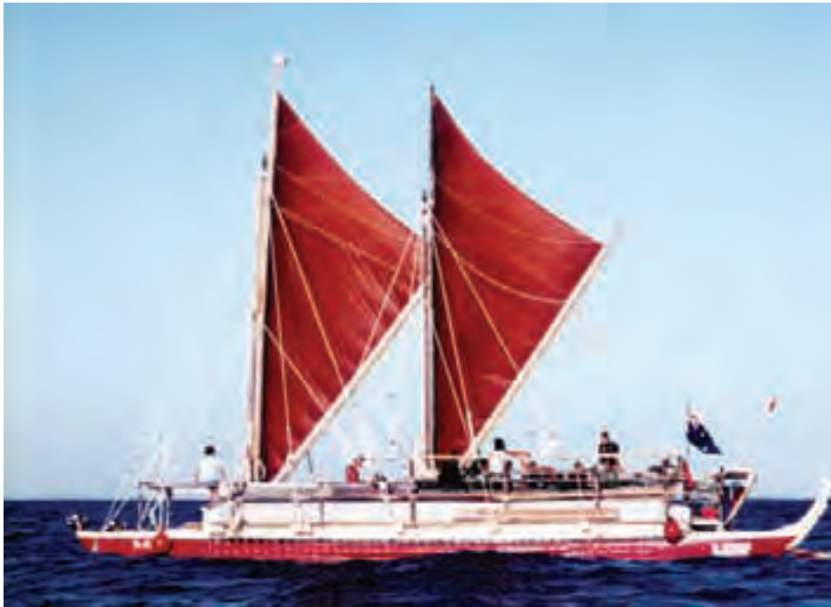
Te Aurere , built by Hekenukumai Busby. This fully functional waka haurua (double-hulled voyaging canoe) is similar to vessels used by early Polynesian voyagers.
